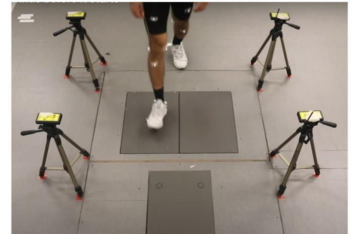
Figure 1. Force plates used to measure vGRF
