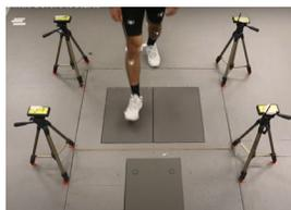
Figure 1. Force Plates used to measure vGRF
