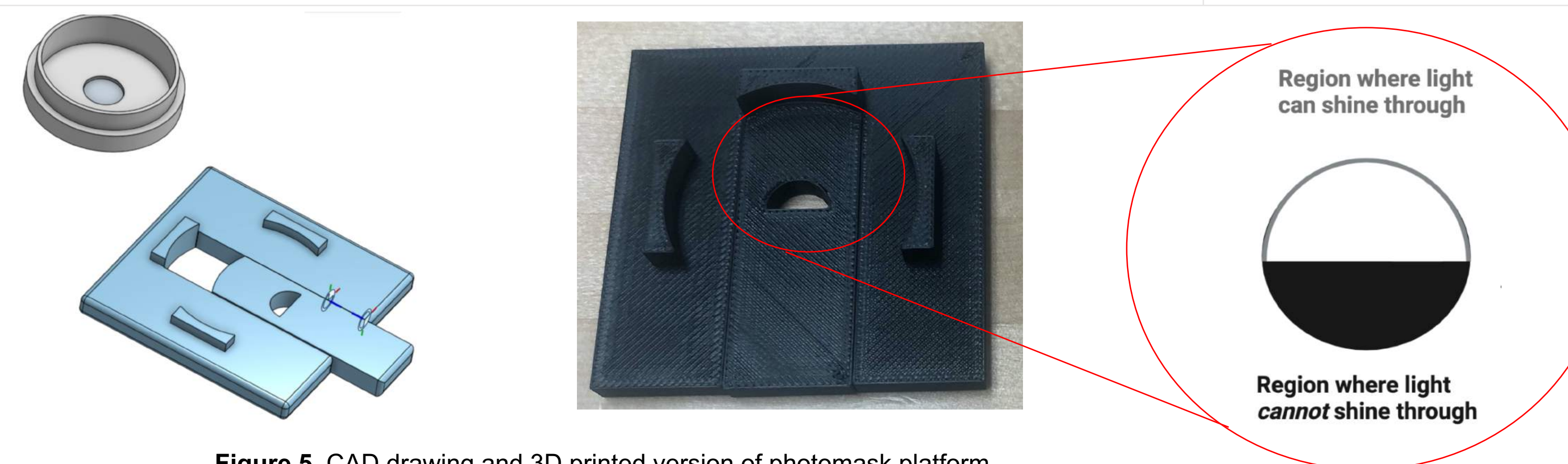
Figure 5. CAD drawing and 3D printed version of photomask platform.
