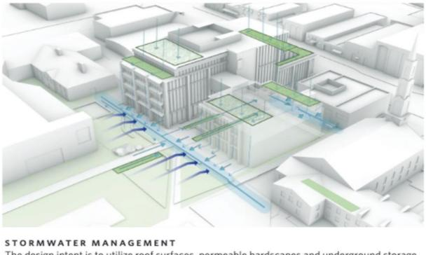
The design intent is to utilize roof surfaces, permeable hardscapes and underground storage for stormwater collection, detention and treatment on a constrained site footprint.
