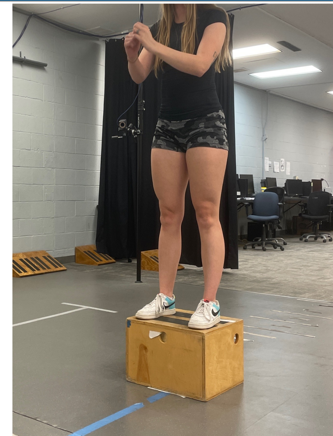
Figure 1. Participants stood on a 30cm tall box that was placed 1/2 their height away from the force plates.
