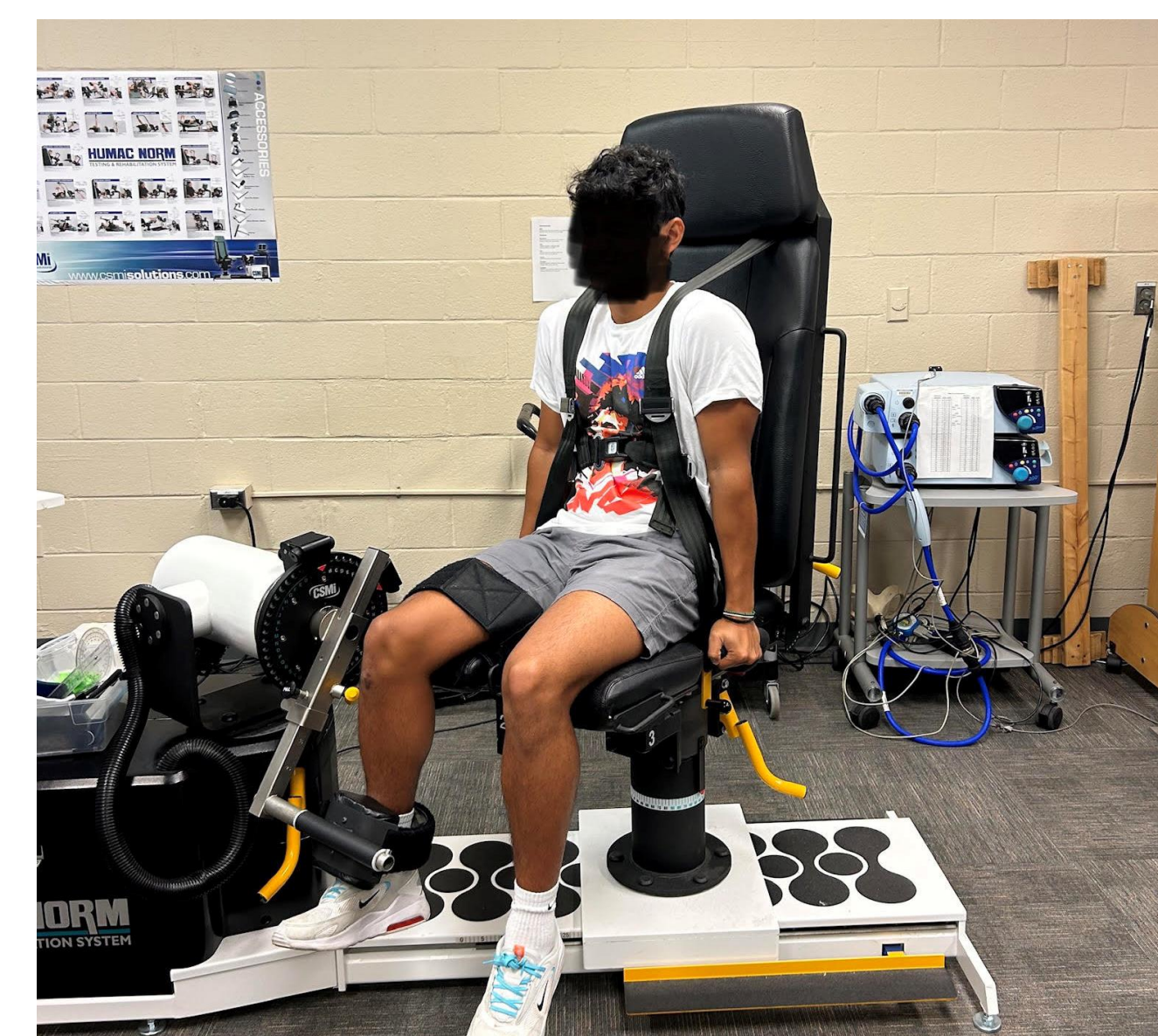
Subjects kicked as hard as they could (left), as the HUMAC dynamometer measured their torque (right)
