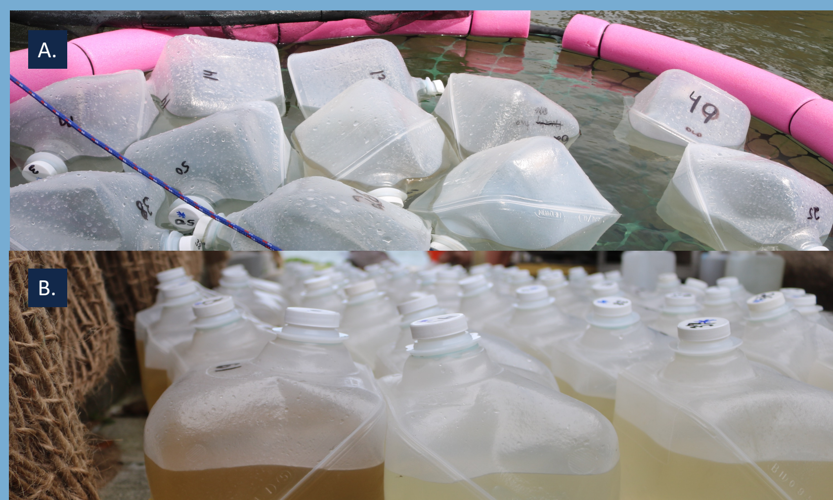
Figure 4. (A). Incubation process of the bioassay. The use of the incubation pool allows for the most similar environmental conditions (temperature and light availability) while experimenting. (B). Cubitainers used for the bioassays. Photo credit: Madison Sholes
