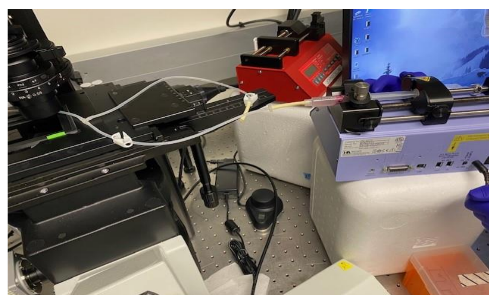
Figure 1: Experimental setup for microfluidic chip analysis. A T connector was used to connect a syringe pump with a dilution of fluorescently labeled microbubbles as well as cell media for flushing to the microfluidic chamber.
