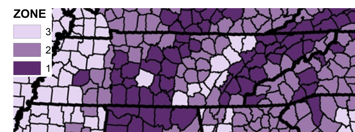
Figure 1: example of county-level resolution US EPA map of GRP radon zones in TN
