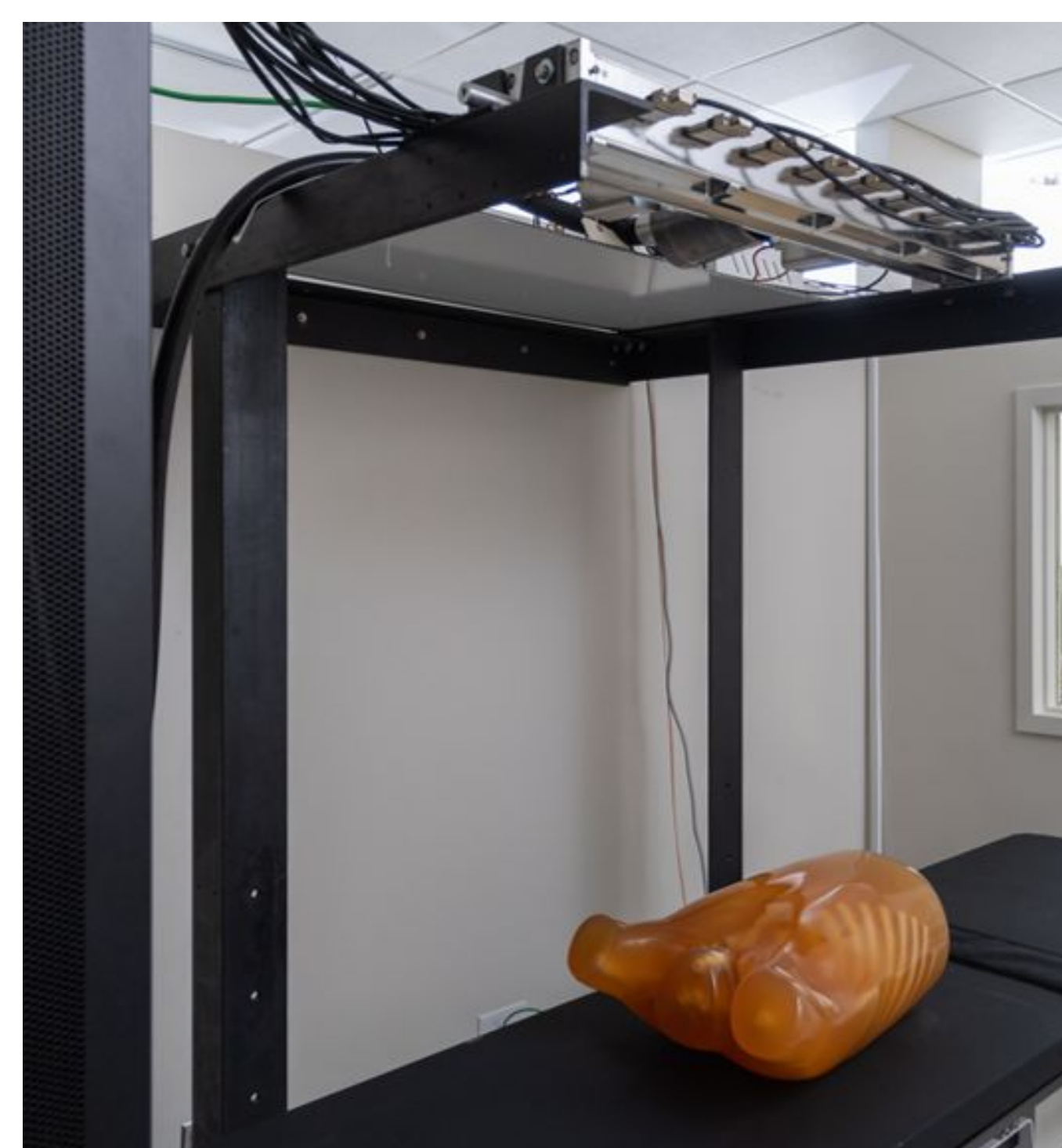
Figure 4. MED1263 CNT x-ray tube in action.
