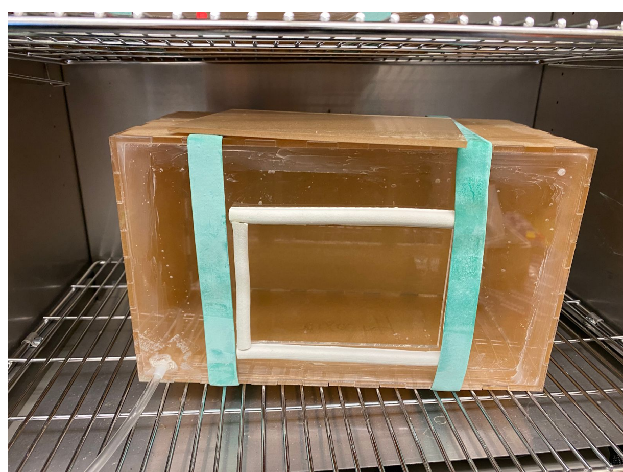
Figure 1: Hypoxia copepod box. A white clear tube supplies nitrogen into the box and is turned on and maintained at 2.5 psi in a controlled temperature environment.
