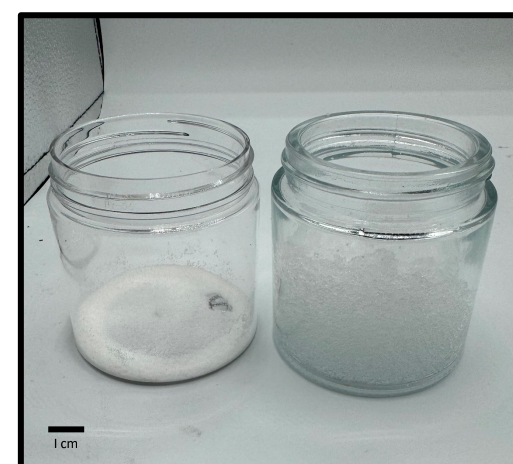
Fig. 6. Image shows the expansion of superabsorbent material from powder state to gel state when water is added.
