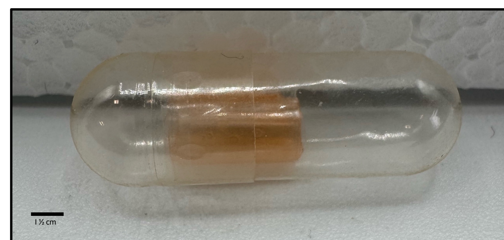
Fig. 2. Image shows a representation of what orally ingestible device will look like inside of the pill capsule.
