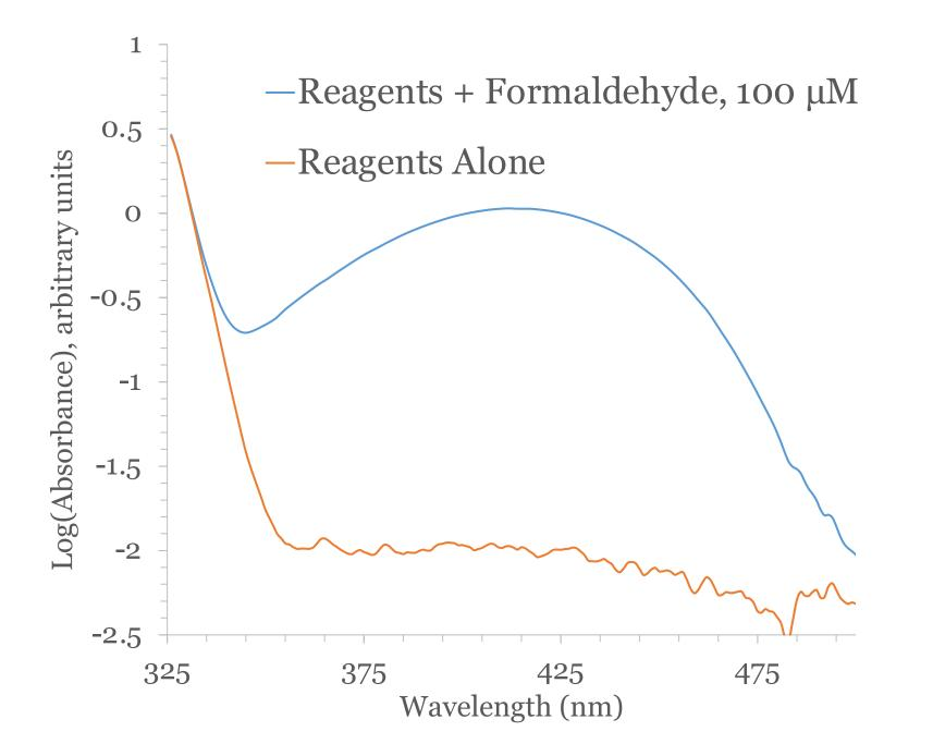
Figure 2. Log absorbance of acetylacetone, ammonium acetate, and acetic acid incubated with and without 10<sup>-4</sup> M formaldehyde, showing smooth  $\lambda_{max}$  = 412 nm in agreement with Nash.<sup>2</sup>
