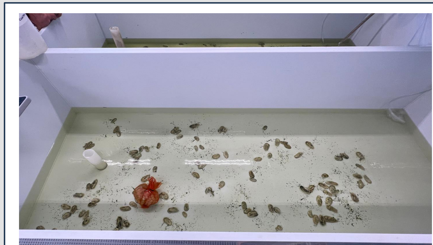
Figure 2. Tank setup with biofilter media bags colonized by denitrifying bacteria.
