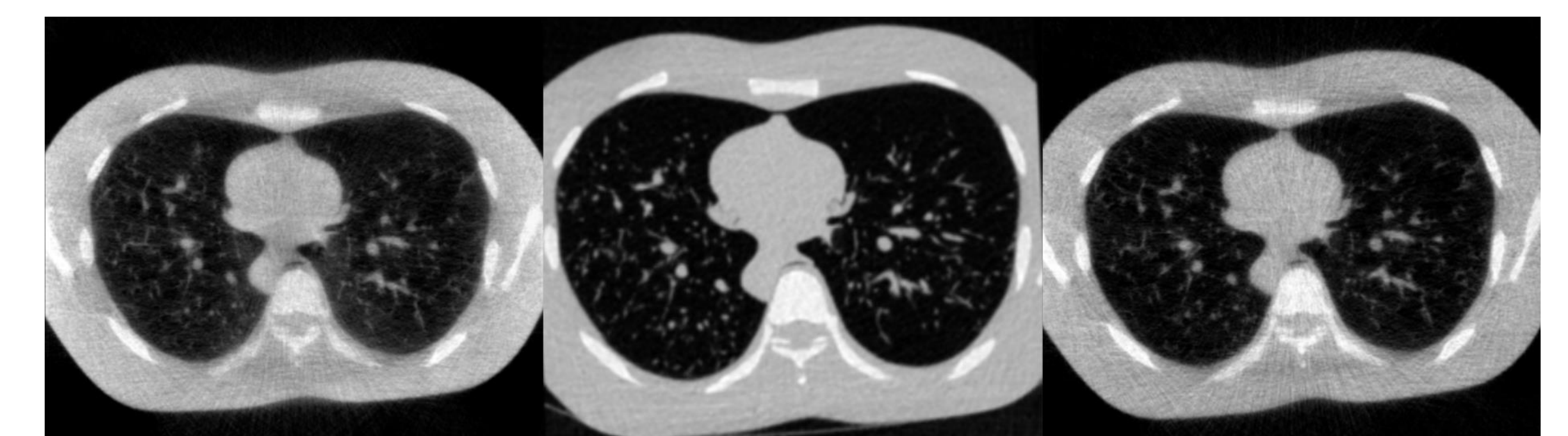
FIG 7. Left: Large angle reconstructed image. Center: clinical CT of same chest phantom for comparison. Right: Small angle reconstructed image
